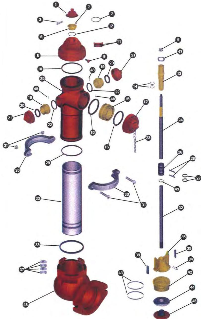
The METROPOLITAN™/M-94 Ductile Iron fire hydrant is a boltless constructed dry barrel traffic model hydrant rated at 250 psi working pressure. It conforms to ANSI/AWWA C502 — AWWA Standard for Dry Barrel Fire Hydrants and is UL Listed and FM Approved.
