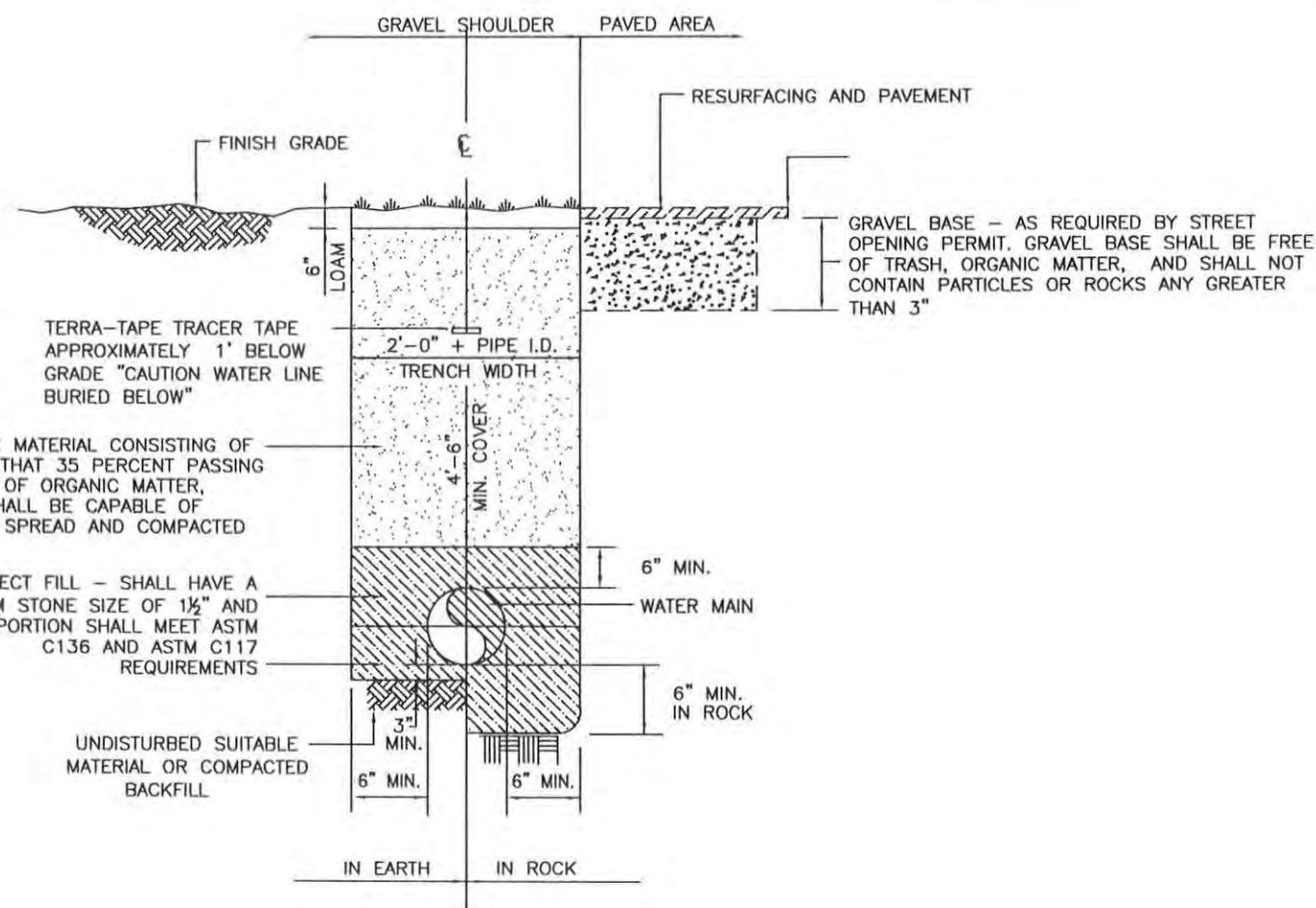
COMMON FILL - SHALL BE GRANULAR MATERIAL CONSISTING OF HARD, SAND AND GRAVEL WITH LESS THAN 35 PERCENT PASSING THE NO. 200 SIEVE. SHALL BE FREE OF ORGANIC MATTER, TRASH, ROOTS, ETC. COMMON FILL SHALL BE CAPABLE OF FORMING A FIRM STABLE BASE WHEN SPREAD AND COMPACTED TO 95%.
